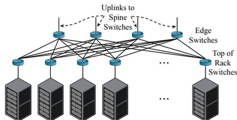
**Figure 10.** Depiction of a server pod, made up of racks and two layers of switches atop, in a Facebook data center [67].
