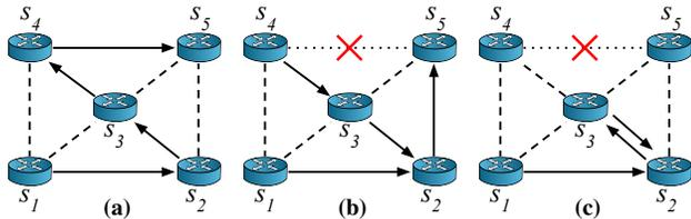
**Figure 2.** (a) The state of the flows to  $s_5$  (b) is planned to be modified by an update to bypass the failure of the  $s_4$ - $s_5$  link but (c)  $s_3$  applies the update before  $s_2$  which creates an unintended network loop.
