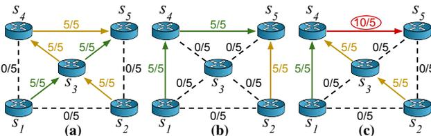
**Figure 3.** (a) The state of the flows to  $s_5$  (b) is planned to be modified by an update alleviating  $s_3$ , (c) but the update is applied by  $s_1$  before it is applied by  $s_2$  which causes an unintended over-provisioning of the  $s_4$ - $s_5$  link.
