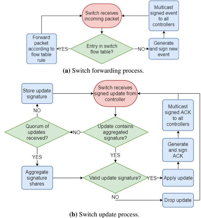
**Figure 6.** Flow charts describing the processes of a switch (a) handling incoming packets on the data plane and (b) handling updates received from the control plane.
