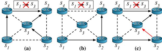
**Figure 1.** (a) The state of the flows from  $s_1$  and  $s_2$  to  $s_5$  (b) is intended to be modified by an update which respects the firewall rule, (c) but  $s_1$  applies the update before  $s_2$  which breaks the firewall rule.
