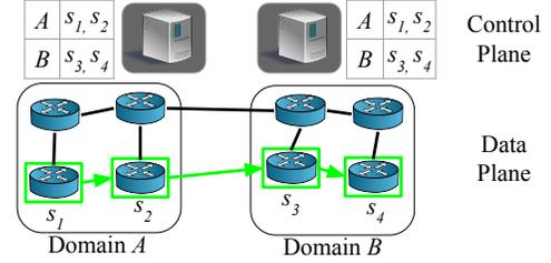
**Figure 5.** Depiction of a two domain network where an event generated by switch  $s_1$  and sent to its local domain control plane. The control plane then uses global domain policies to determine that network updates involve both domains  $A$  and  $B$ . The control plane of  $A$  forwards the event to  $B$  and both domains update their local switches to set flow tables rules.
