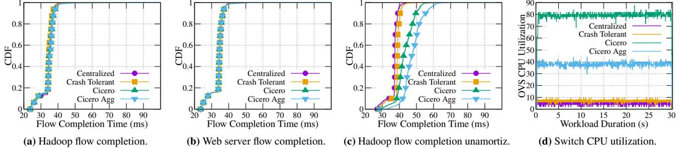
**Figure 11.** Cicero performance on a single-domain network comparing a centralized solution to a control plane, made of 4 controller replicas, that uses either a crash-tolerant update protocol, Cicero without/with controller aggregation. (a) and (b) depict the CDF of Hadoop and web server flow completion times, respectively. (c) depicts the CDF of Hadoop flow completion times when routes are removed upon flow completion. (d) depicts the (switch) CPU utilization of OVS during a Hadoop workload.
