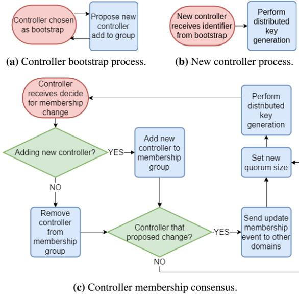
**Figure 8.** Flow charts for controller membership change: (a) and (b) show the processes for the bootstrap controller and the joining controller respectively, and (c) shows the controller process when a membership change consensus is reached.
