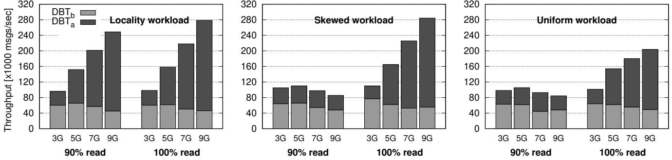
(b) Effect of dynamic access on throughput with increasing number of replicas.
