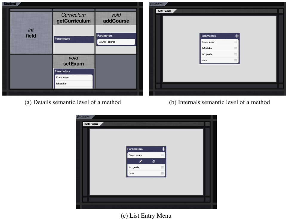
Figure 4.14. The internals of a method: parameters' visualization
