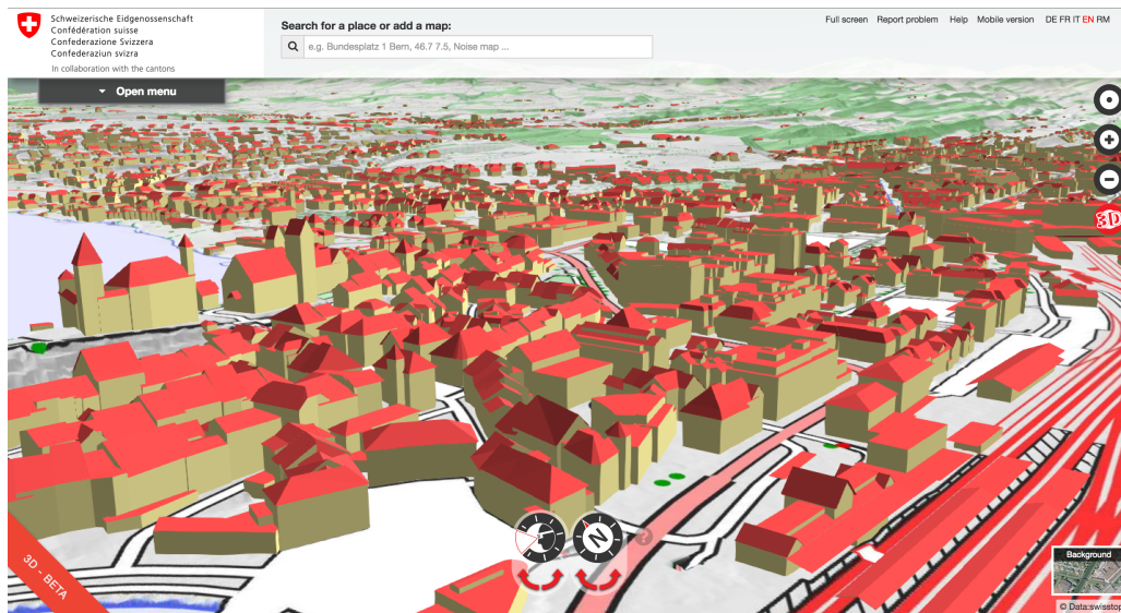
Figure 2.8. A 3D visualization of the city of Bern in the Swiss Geospatial Portal. Using Cesium 3D Tiles Technology
