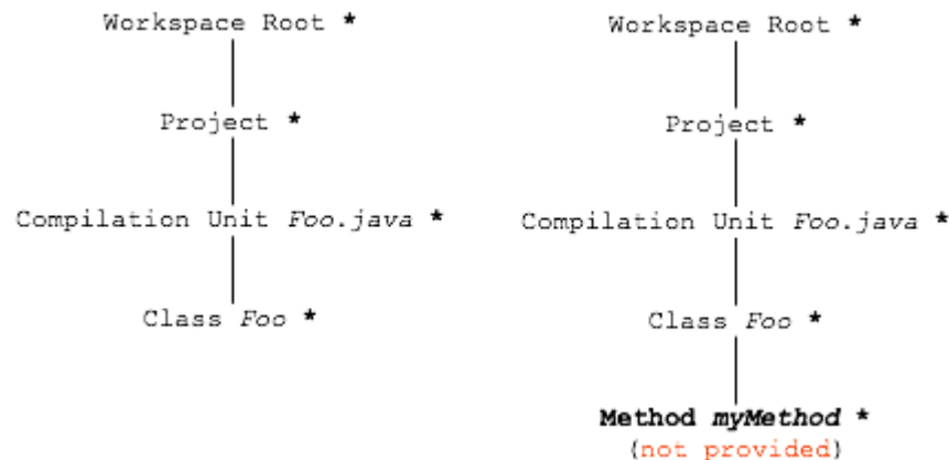
Figure 3.3: Example of a java delta tree for method modification
