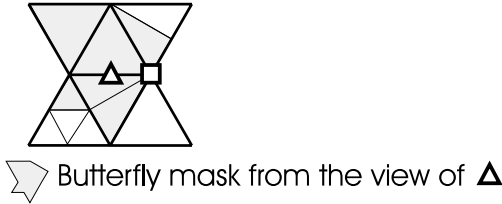
Figure 12: After a split in the Butterfly mask of an odd vertex \triangle has been performed this mask is no longer given by the three neighboring triangles above and the three ones below the split edge (cf. Fig. 2).
