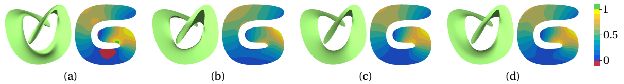
Figure 1: Interpolants of height data (ranging from 0 to 1) given at the boundary of a non-convex planar domain, based on transfinite mean value (a), positive Gordon–Wixom (b), harmonic (c), and our novel transfinite barycentric coordinates (d). The left images show a 3D view of each interpolant, the right images an orthographic projection from above. Height values in the intervals [k, k + 1]/10 for k = -1, 0, \dots, 10 are colour-coded as indicated by the colour bar, with negative values in red, values above 1 in green, and values between 0 and 1 in colours from blue to yellow.
