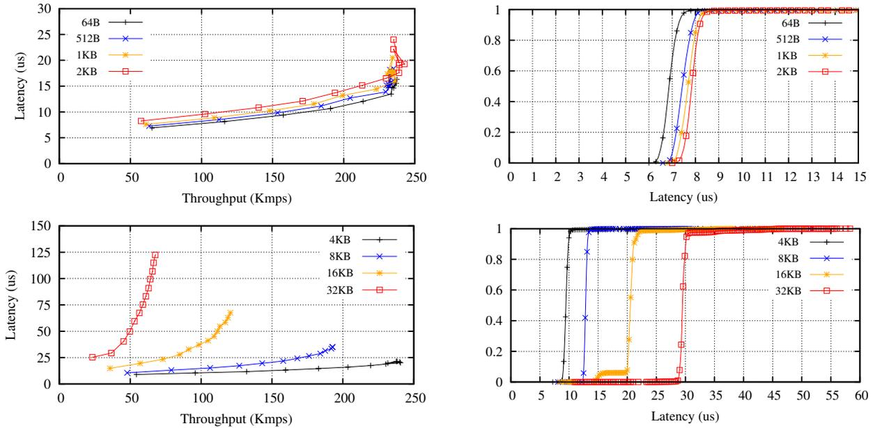
**Figure 4: RamCast performance with different message sizes: 64B to 2 KB (top) and 4 KB to 32 KB (bottom), throughput versus latency (left) and latency cumulative distribution function for a single client (right).**
