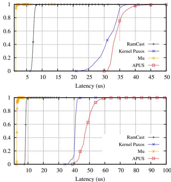
**Figure 6: Latency cumulative distribution function for RamCast and atomic broadcast protocols with a single client: 64-byte messages (top) and 1K-byte messages (bottom).**
