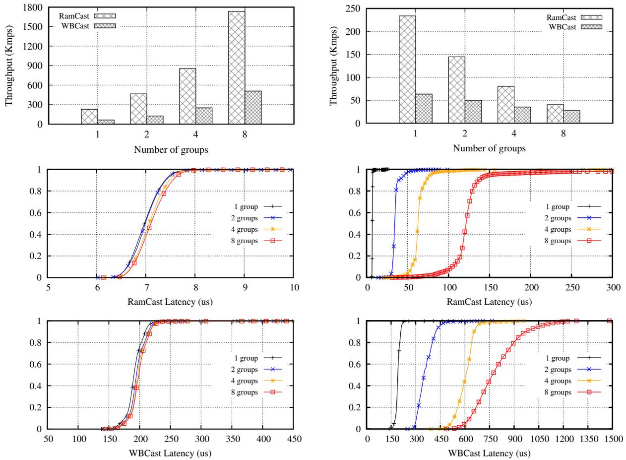
**Figure 5: Performance of atomic multicast when messages are multicast to a single group (graphs on the left) and to all groups (graphs on the right). In each case, we show: throughput (top) and latency cumulative distribution function with one client for RamCast (middle) and WBCast (bottom).**
