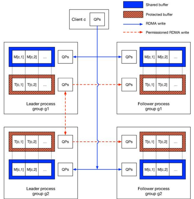
**Figure 2: RamCast’s memory layout. The normal execution proceeds in three steps: in step 1, the client writes a multicast message in the memory of all destination processes; in step 2 the leader of each destination group proposes and writes a timestamp for the message in the memory of its followers and other leaders; in step 3 the leaders propagate the timestamp written by other leaders, and the followers acknowledge the proposed timestamps. The message is delivered after step 3.**
