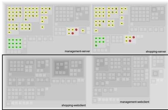
Fig. 4. Separation of concerns in Veniqa , between backend (top) and frontend (bottom) microservices.
