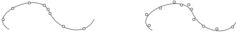
Figure 7: The configuration to the left is suitable for interpolation while approximation should be used for the noisy data points to the right.
