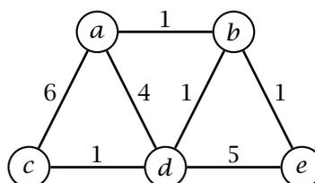
Write the first iterations of the distance-vector routing algorithm until the protocol converges to a stable state. For each iteration, list the routing tables of each router. (20')
