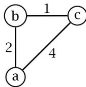
For simplicity, assume all routers start at time 0, that routing messages (i.e., distance vectors) are sent out by routers every 10 seconds, and that they are received by neighbor routers after one second. Write the first iterations of the distance-vector routing algorithm, at times 0, 10, ..., until the protocol converges to a stable state. For each iteration, list the routing tables of each router. (15')
