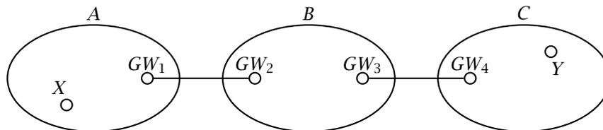
Illustrate the idea of hierarchical routing in the particular case of the Internet by describing the process by which an IP packet would be routed from a source router *X* in *A* to a destination router *Y* in *C*. For each step, briefly discuss which routing information is used, which protocol determines that routing information, and how that routing information is transmitted to the router. (10')
