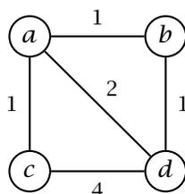
Assuming that routers exchange routing information synchronously (at the same time), illustrate the state of each router until the routing protocol stabilizes. (25')
