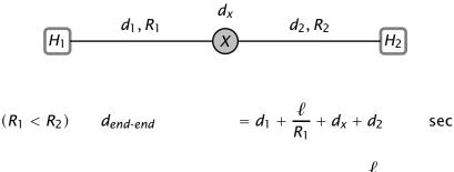
$(R_1 \ge R_2)$   $d_{end-end} = d_1 + d_x + d_2 + \frac{\ell}{R_2}$  sec
