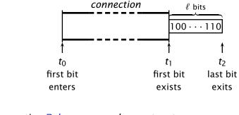
Propagation Delay  $d_{prop} = t_1 - t_0$  sec
