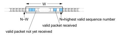
Receiver must keep track of a fixed window of packets (fixed size W, at least W = 32, default W = 64)
