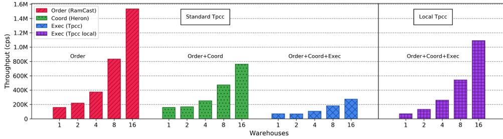
Figure 5.2. Performance of RamCast, Heron, TPCC, and TPCC local with increasing number of partitions.
