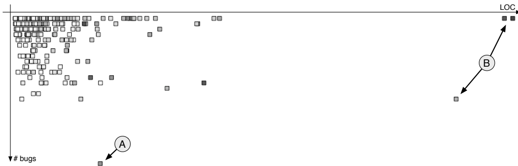
Figure A.2. A Correlation view applied to the ArgoUML software system. Nodes represent classes, nodes' position represents number of lines of code (x) and number of post-release bugs (y), and nodes' color maps the number of methods.
