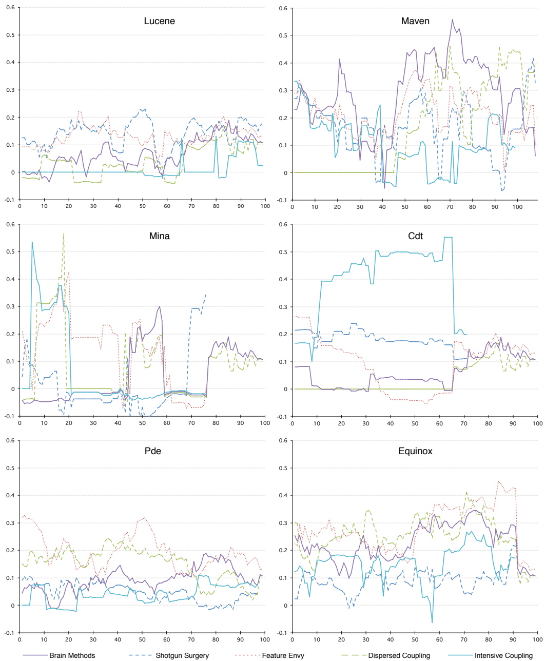
Figure 10.5. Spearman's correlations between number of design flaws and number of post-release defects over multiple versions of software systems
