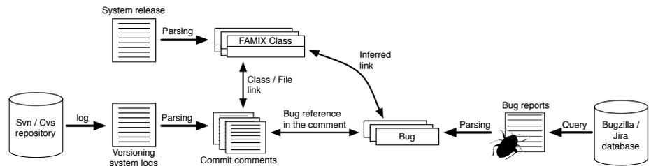
**Fig. 3.** Linking bugs, SCM files and classes.
