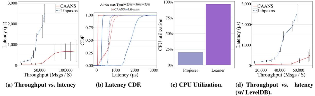
**Figure 7: The end-to-end performance of CAANS compared to libpaxos: (a) throughput vs. latency without, (b) latency CDF, (c) CAANS CPU Utilization, and (d) throughput vs. latency with LevelDB. CAANS demonstrates higher throughput, lower latency, and more predictable latency. Moreover, CAANS moves the processing bottleneck to the learner component, suggesting that even better performance should be possible.**
