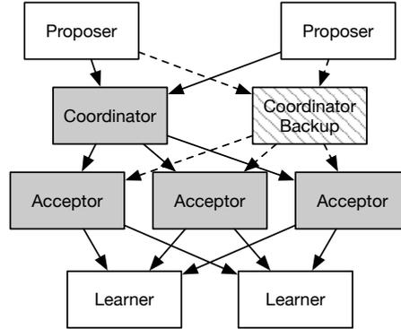
**Figure 3: A switch-based deployment of CAANS. Switch hardware is shaded grey, and commodity servers are colored white. The arrows represent communication. The coordinator backup may be deployed on either switch hardware or a commodity server. The dashed-arrows represent backup communication.**
