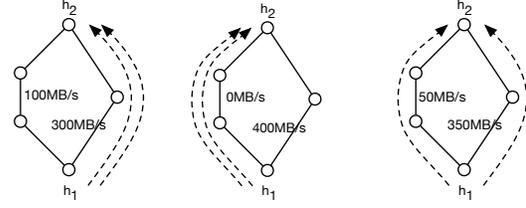
(a) Shortest-Path (b) Min-Max Ratio (c) Min-Max Reserved
