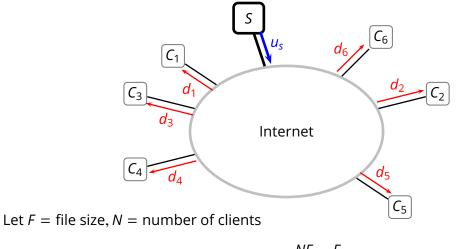
$$T_{CS} \ge \max\left(\frac{NF}{u_s}, \frac{F}{d_{min}}\right)$$
