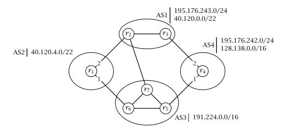
*Question 1:* Indicate (on the figure) which connections are eBGP and which ones are iBGP.
