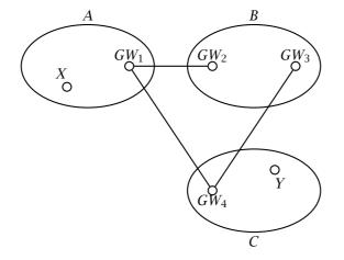
Illustrate the idea of hierarchical routing in the particular case of the Internet by describing the process by which an IP packet would be routed from a source router X in A to a destination router Y in C. For each step, briefly discuss which routing information is used, which protocol determines that routing information, and how that routing information is transmitted to the router.
