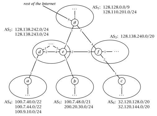
Write the forwarding tables of all the seven routers, using the actual IP prefixes and the interface numbers annotated in the figure. Routing must be follow shortest paths, and addresses must be combined ("supernetting") whenever possible. Make sure all addresses are correctly reachable, including all addresses in the rest of the network.
