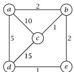
In the initial state each router knows the costs of the links to its neighbors. Assuming that routers exchange distance vectors in a synchronous way (i.e., all at the same time) show the state of router *a* after each update to its routing tables until the protocol converges.
