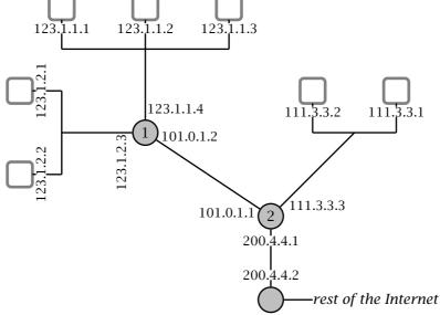
Write the forwarding tables of routers 1 and 2. Assume longest-prefix matching. Assume also that each subnet holds a block of 256 addresses. In writing the forwarding tables, identify each output port directly with their IP address.
