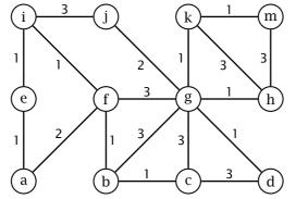
*Question 1:* Write all the routing information maintained by router f at a time when the routing protocol has converged to a stable state. (Hint: this includes router f's distance vector as well as the distance vectors received from its neighbors.)
