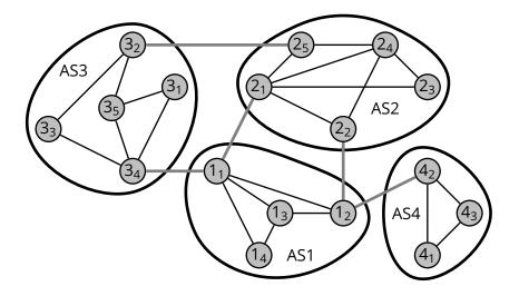
An inter-autonomous system routing protocol determines routing at the autonomous-system level
